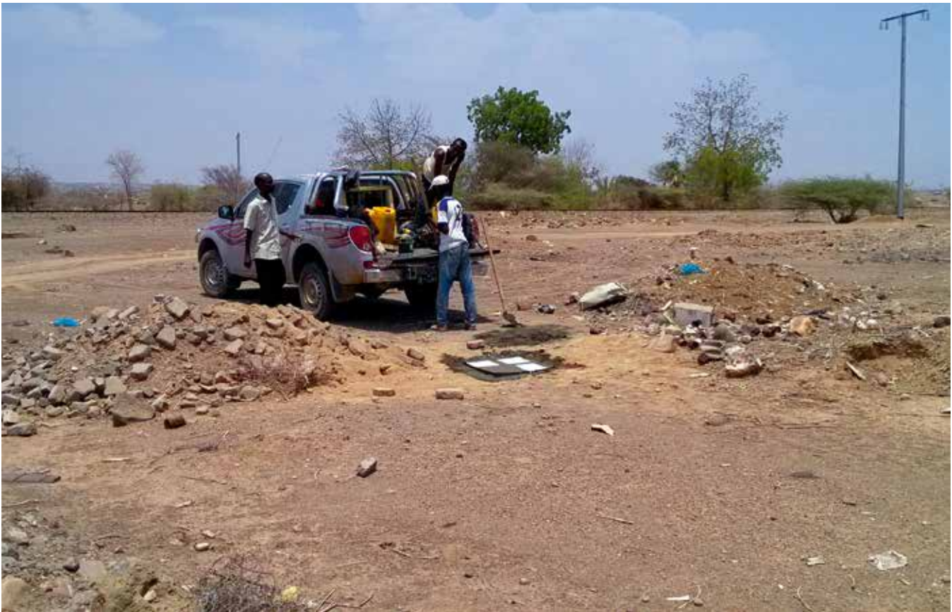
Marking and surveying ground control points with GPS
